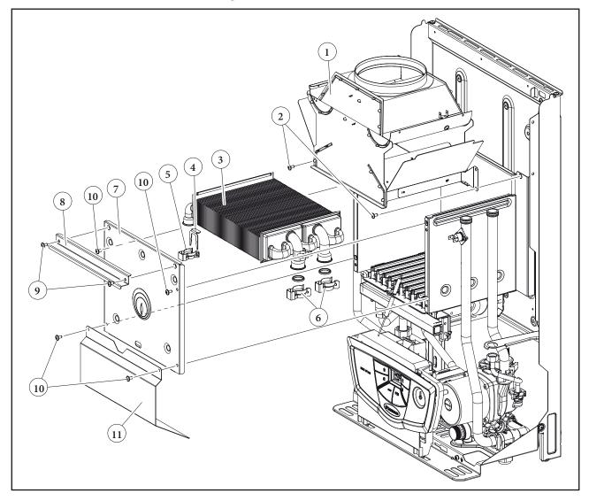
Before disassembling the components, make sure that the gas cock is closed and empty the CH system and the DHW circuit.
