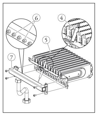
**Note:** for correct ignition and detection of the boiler always respect the quotes stated in the figure below.
