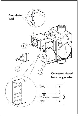
It acts on the gas valve stabiliser and allows the variation of the outlet pressure proportionally to the direct current that passes through it.
