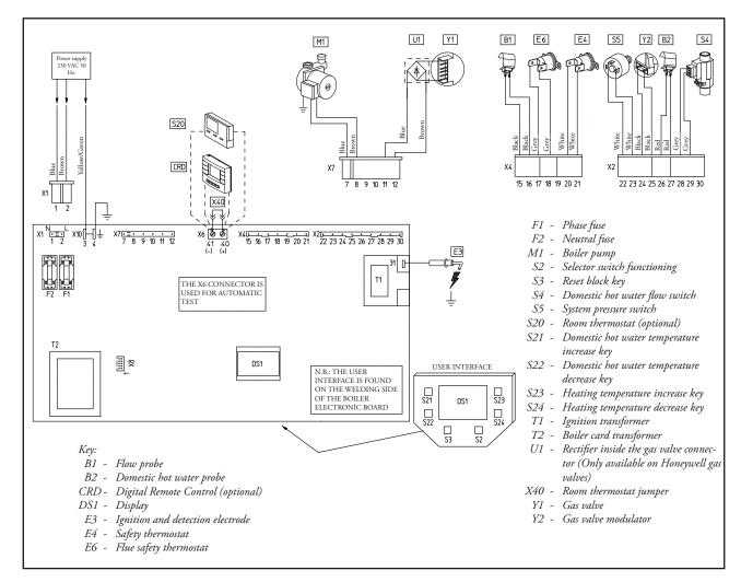
The electric circuit of the NIKE Star 24 3 E is completely interlocked to a P.C.B. with integrated microprocessor, which controls the functions of the generator.
