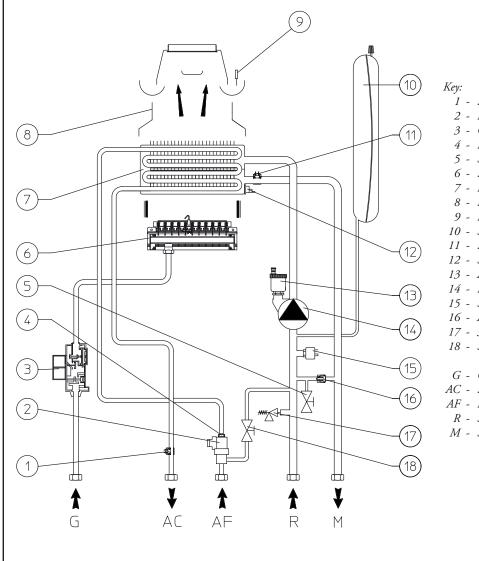
The hot water used for central heating and domestic hot water is produced thanks to two distinct circuits that are affected according to necessity.
