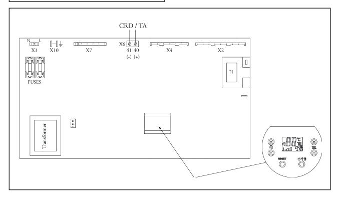
Inside the control panel the boiler is equipped with a P.C.B. with microprocessor for control of the appliance's electric devices, which takes care of linear modulation of burner power.
